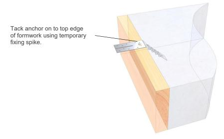
2. After initial concrete cure, position wall frame. Bend anchor up and fix 2 nails into edge.
