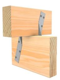
• Ceiling and Purlin Hangers installed on opposing corners using 2 x LH, fixed with 3 nails option to each leg per hanger. Hanger installed in PAIRS.
