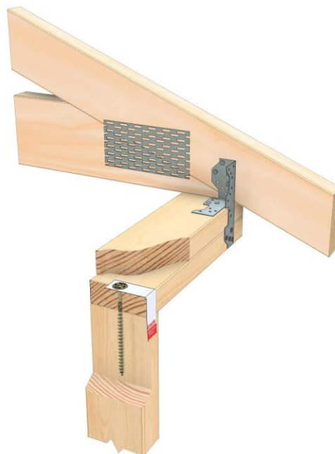
Pryda Screw used with Long Multigrip secured to top plate. 135mm screw installed through top plate only.
