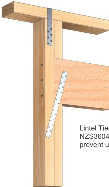
Top plate to stud Tie-down with strap wrapped over plate.
