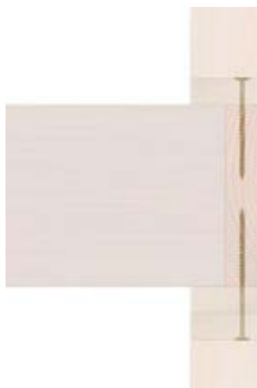
Single 45mm wall plate into side grain.
