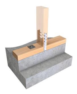
Stud to bottom plate Tie-down to NZS3604:2011 Figure 8.12 to prevent uplift.
