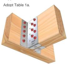
All screws shown are Pryda Timber Connector Screws. Black Head = 65mm length. Red head = 35mm length.
