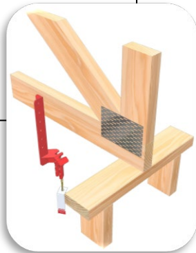
Truss standard heel to top plate
